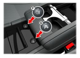
*[F] REAR FOG LAMPS:* Used with the dipped beam when fog or mist is causing restricted visibility. They **must** be set to OFF when visibility clears to reduce glare to the drivers of following vehicles.
