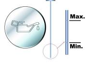
Approximately one litre is required to bring the level from Min. to Max.
