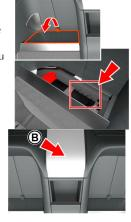
7. With a person each side, support the tonneau lid in the fully raised position, while raising the roof. Place one hand under the roof lining and the other hand under the roof tension bow (positions shown) - lift, both sides, until the tension bow clears the tonneau lid.
