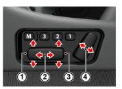
The seat must be moved to its limit of travel and allowed to stall for 1 second for each axis. If the seat is not held at its limit of travel. the seat memory will not learn this as its fully travelled position.
