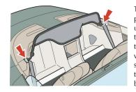
To remove the wind deflector pull up at the points shown to un-clip the two tabs from the top seat belt mounts. Remove the wind deflector from the vehicle, fold it flat, put it in the storage bag and place the bag in the storage area in the vehicle boot.
