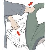
Hold the roof in position while the tonneau lid lowers.
