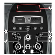
[1] VOLUME/ON/OFF: Volume control. Press to mute the audio system. Press and hold to turn the infotainment screen on or off.
