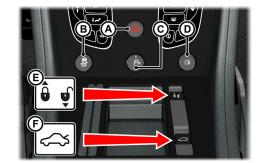
**[A] HAZARD WARNING LAMP:** Press to set the hazard warning lamps to ON or OFF.
