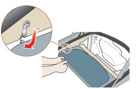
Keep the rear section folded and turn the boot cover 180°. Place the cover in the rear section of the boot.
