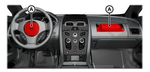
The front airbags (A) only deploy in a serious front collision. The side airbags<sub>1</sub>, located in the front seats (B) only deploy according to which side has been impacted in a serious side collision.
