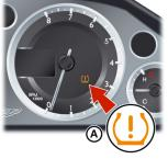
showing which tyre(s) have low or high air pressure and the current tyre pressure. When the tyre pressure indicator comes ON, stop and check your tyres as soon as possible, and inflate or deflate them to the correct pressure.
