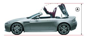
If the vehicle is moving while the roof is being raised or lowered, roof movement will continue, while the roof switch is pressed, until the roof has locked in the raised or lowered position.
