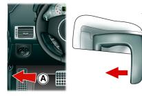
Pull the bonnet release lever (A) located in the left front footwell. The Slightly lift the front edge of the bonnet whilst pulling upward on the open. The bonnet is held open by two gas struts.
