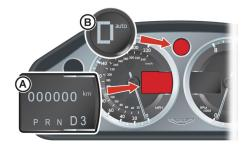
Kick-down is used in circumstances where rapid acceleration is required, i.e. when overtaking. Kick-down is when the accelerator pedal is quickly depressed, causing the transmission to change down to the lowest gear possible to achieve maximum acceleration. The gear engaged depends on the road speed at the time of kick-down.
