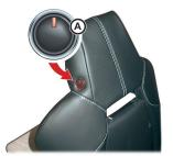
In the unlikely event of power failure, a manual release strap is provided in the seat back. Pull and hold the strap to release the seat back and then move the seat back forward.
