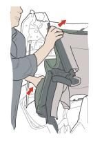
8. When the rear tension bow has cleared the tonneau lid, let the tonneau lid lower.
