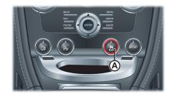
**TRACK MODE:** Press and hold the DSC button (A) for four seconds and release. DSC TRACK MODE SELECTED will show in the message centre (right). This raises the thresholds at which the DSC system operates. While the DSC system operates to correct the vehicle stability the DSC symbol will flash.
