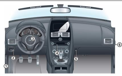
[1] FUEL FLAP RELEASE: Press to open the fuel flap. Close the fuel flap by pressing down on the flap until the lock engages.
