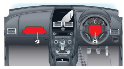
The front airbags (A) only deploy in a serious front collision. The side airbags<sub>1</sub>, located in the front seats (B) only deploy according to which side has been impacted in a serious side collision.
