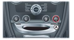
At engine start Sport mode will be OFF by default. Press the Sport button (A) once to enter Sport mode (button LED ON) and press again to exit.
