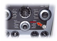
♥ If the vehicle has not been locked or unlocked and the mirrors have been folded using the power fold function then the mirrors will stay folded until placed in the driving position using the power fold function again.
