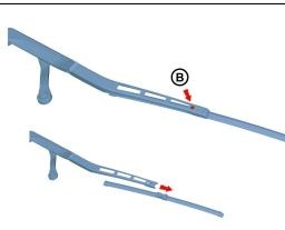
After replacing the wiper blade either:
