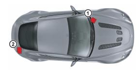
[1]: Engine bay fuse box (passenger side).[2]: Boot fuse box.
