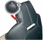
L In the unlikely event of power failure a manual release strap is provided in the seat back. Pull and hold the strap to release the seat back and then move the seat back forward.
