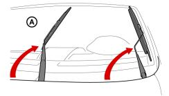
Lift the wiper arm(s) up, press at point B and remove the worn wiper blade(s). Install the new wiper blade(s) and lower the wiper arm(s).
