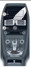
[1] SATELLITE NAVIGATION SCREEN<sub>1</sub>: Opens when the Satellite Navigation system is set to ON(Refer to 'Satellite Navigation', page 9.1).
