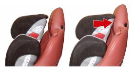
Motor the passenger seat fully to the rear and install the Britax 'Evolva 2-3 ISOFIT' child seat to the passenger seat ISOFIX bars as per the manufactures instructions. Adjust the height of the child seat headrest as required according to manufactures instructions. Tilt the passenger seat back forward until the top of the child seat comes into contact with the passenger seat - as shown.
