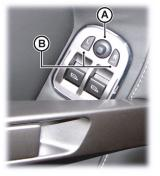
When the heated rear window is ON the heaters in the door mirrors will operate for 6.5 minutes.
