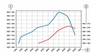
[1]: Torque (Nm / lb/ft) [2] : Power (kw / bhp) [3]: Engine speed (rpm)
