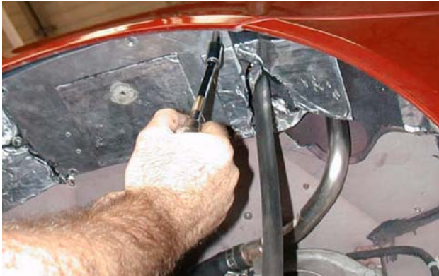
6. Disconnect two wiring harness plugs.
