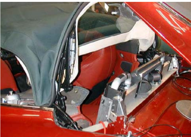
8. Remove the rollbar trim cover.
