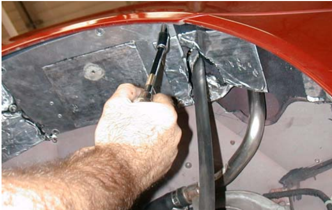
6. Disconnect two wiring harness plugs.
