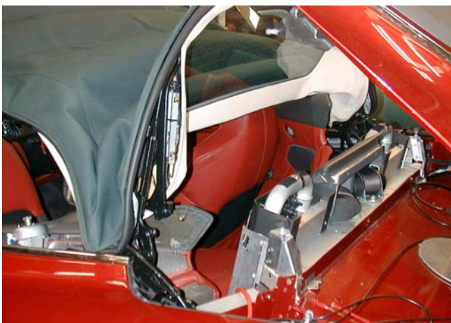
8. Remove the rollbar trim cover.
